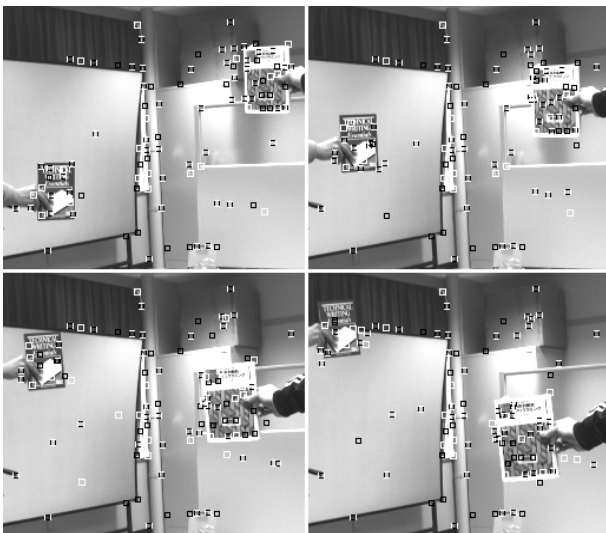
Figure 3: Image sequence and feature points for 3D reconstruction, 1st frame(upper left), 10th frame(upper right), 20th frame(lower left), and 30th frame(lower right).
