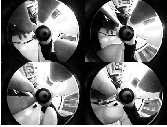
Figure 2. Typical image frames obtained by omnidirection camera with fingers. Upper-left:begin with three fingers, upper-right:changed to two fingers, lower-left:four fingers, and lower-right:three fingers again. Tapping of finger is also a typical motion of fingers.
